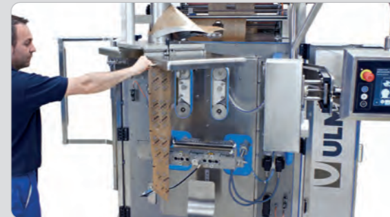
Possibility of changing format on one side: practical, safe, ergonomic and simple.
