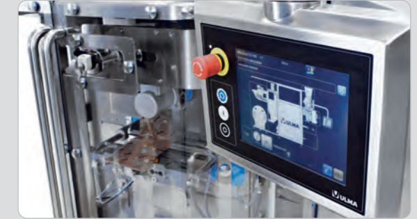
Control by 10" industrial PC touch screen: screen integrated features (production data, test screen, machine manuals, videos, driver download...).
