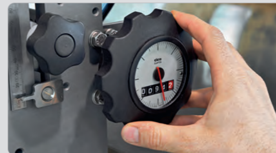
Easy to use for the machine operator: simplified daily adjustments without tools.
